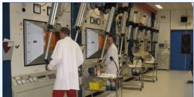
Figure 2.  $^{99}\text{Mo}$  production in hot cells at the company's facility in Petten.
