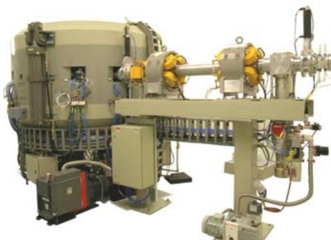
Figure 1. An 18 MeV cyclotron (IBA Cyclone®) with beam line for solid target. This equipment could be adapted to produce  $^{99m}\text{Tc}$  provided it is cost-effective.
